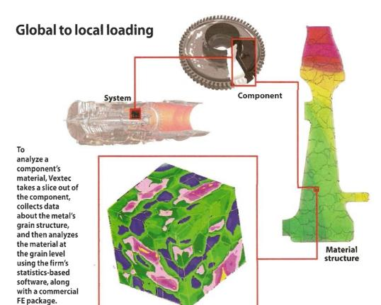
A managed service and software with a statistical basis links to FE to model part failure at the grain level.
